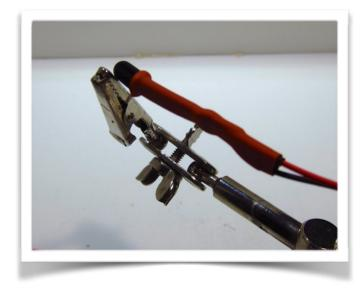
Put the larger heat shrink over the whole assembly from the LED down. Don't cover the LED or it won't fit inside the sensor plastics.
