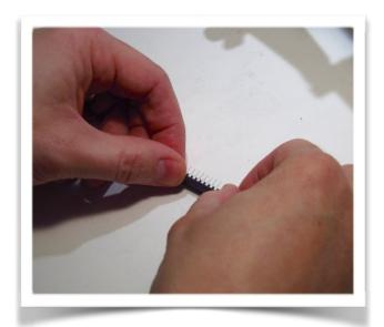
Grip the chip gently with both hands and press the pins on a flat surface, gently rolling the chip up until it's perpendicular with the table. Turn it over and do the same for the other side. Move it only a little at a time. It's better to do it again and add a little more adjustment than to undo it entirely if pins get tilted inwards.
