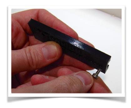
The front piece is printed with the XTension name and has a channel for the wire from the sensor on its back. Start the 2 screws by hand into the plastic until they are just flush with the back of the plastics.
