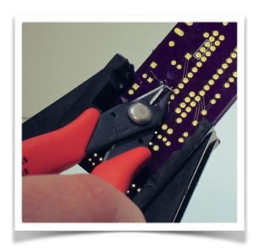
Step 3: Install Capacitor C7
