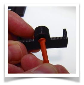
Insert the phototransistor from the back of the clip and bend the wires so that they fall straight down as in this picture's orientation. Apply some hot glue or other sealant and press on the cap which will cover the back of the phototransistor and protect the bend in the wires.
