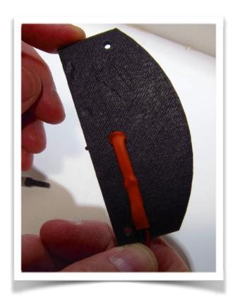
Bend the leads to whichever side more easily reaches the radio/CPU installation.
