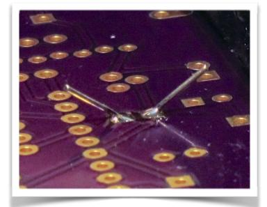
When you're done, you want to see something like this. The puddle of solder is firmly attached to the pads on the board, not sitting on top like a ball, and has drawn up around the leads a little. There are no messy edges or blobs and no solder is touching any adjacent pads.
